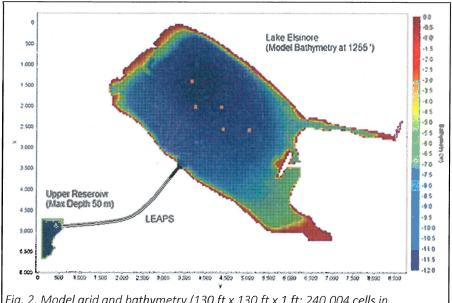
Fig. 2. Model grid and bathymetry (130 ft  $\times$  130 ft  $\times$  1 ft; 240,004 cells in computational domain at full pool). Axial flow pumps depicted as brown squares, approximate location of diffused aeration lines shown as light purple lines.
